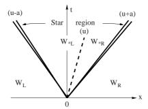
Fig. 4.1. Structure of the solution of the Riemann problem on the x-t plane for the one–dimensional time–dependent Euler equations
