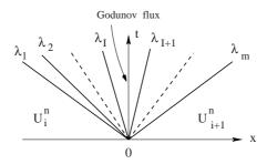
Fig. 5.8. Evaluation of the Godunov intercell flux for linear hyperbolic systems with constant coefficients
