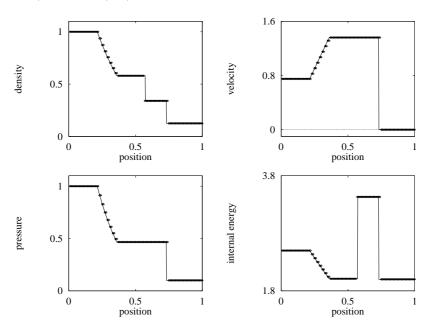
Fig. 7.14. Lax–Friedrichs Random Choice scheme applied to Test 1, with  $x_0 = 0.3$ . Numerical (symbol) and exact (line) solutions are compared at time 0.2 units
