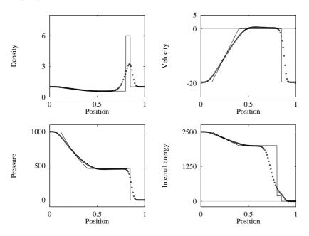
Fig. 7.22. FORCE scheme applied to Test 5, with  $x_0 = 0.8$ . Numerical (symbol) and exact (line) solutions are compared at the output time 0.012 units
