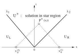
**Fig. 2.5.** Structure of the solution of the Riemann problem for a  $2 \times 2$  linear system with constant coefficients
