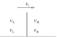
Fig. 2.18. Illustration of the Rankine–Hugoniot conditions for a single discontinuity of speed  $S_i$  connecting two constant states  $\mathbf{U}_{\mathrm{L}}$  and  $\mathbf{U}_{\mathrm{R}}$  via a system of conservation laws
