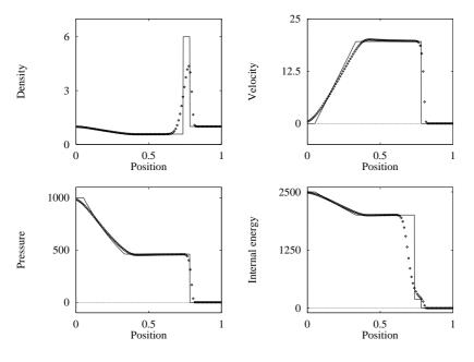
Fig. 6.10. Godunov's method applied to Test 3, with  $x_0 = 0.5$ . Numerical (symbol) and exact (line) solutions are compared at the output time 0.012 units
