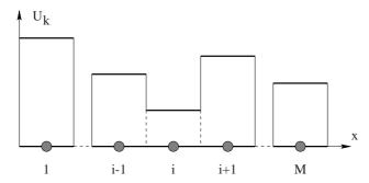
Fig. 6.1. Piece—wise constant distribution of data at time level n, for a single component of the vector  ${\bf U}$
