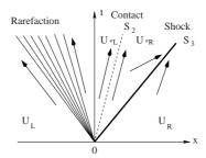
**Fig. 3.2.** Structure of the solution of the Riemann problem in the x-t plane for the time-dependent, one dimensional Euler equations, in which the left wave is a rarefaction, the middle wave is a contact discontinuity and the right wave is a shock wave
