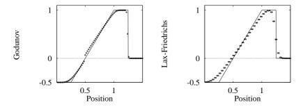
Fig. 5.15. Test 3: Inviscid Burgers's equation. Comparison of numerical results for two schemes (symbols) with the exact solution (line) at time 0.5 units (32 time steps)
