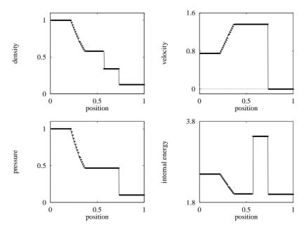
**Fig. 7.10.** Random Choice Method applied to Test 1, with  $x_0 = 0.3$ . Numerical (symbol) and exact (line) solutions are compared at the output time 0.2 units
