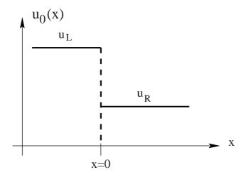
**Fig. 2.2.** Illustration of the initial data for the Riemann problem. At the initial time the data consists of two constant states separated by a discontinuity at x = 0
