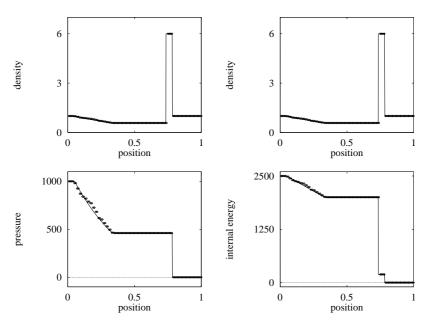
Fig. 7.16. Lax–Friedrichs Random Choice scheme applied to Test 3, with  $x_0 = 0.5$ . Numerical (symbol) and exact (line) solutions are compared at time 0.012 units
