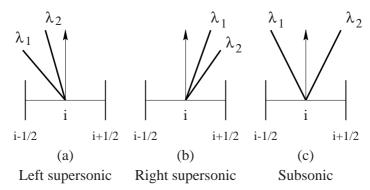
**Fig. 8.2.** Possible flow patterns in cell  $I_i$  at time n: (a) supersonic flow to the left (b) supersonic flow to the right (c) subsonic flow
