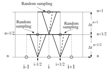
Fig. 7.8. Illustration of the Random Choice Method, on a staggered grid
