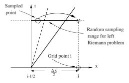
Fig. 7.5. RCM sampling of the right-hand side of the left Riemann problem solution, when  $0 \le \theta^n \le \frac{1}{2}$ . Sampled state is assigned to the centre of cell  $I_i$
