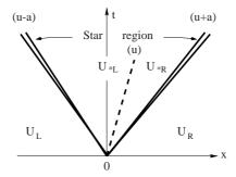
**Fig. 3.1.** Structure of the solution of the Riemann problem in the x-t plane for the time-dependent, one dimensional Euler equations. There are three wave families associated with the eigenvalues u - a, u and u + a
