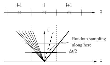
Fig. 7.7. Random choice scheme of the Lax–Friedrichs type for non–linear systems. Updated solution in cell  $I_i$  at time  $\Delta t$  is obtained from random sampling solution of Riemann problem  $RP(\mathbf{U}_{i-1}^n, \mathbf{U}_{i+1}^n)$  at time  $\frac{1}{2}\Delta t$
