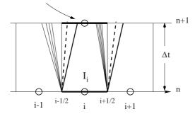
Fig. 7.4. The RCM on non-staggered grid. Solution is updated to time level n by random sampling solutions of Riemann problems within cell  $I_i$  at time  $\Delta t$
