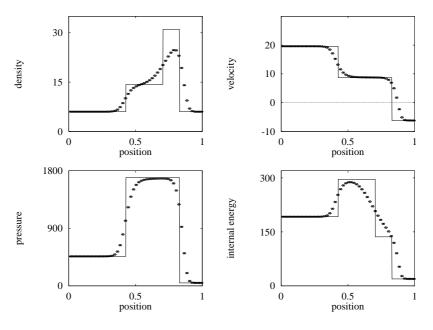
Fig. 6.16. The Lax–Friedrichs method applied to Test 4, with  $x_0 = 0.4$ . Numerical (symbol) and exact (line) solutions are compared at the output time 0.035 units
