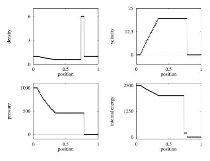
Fig. 7.12. Random Choice Method applied to Test 3, with  $x_0 = 0.5$ . Numerical (symbol) and exact (line) solutions are compared at the output time 0.012 units
