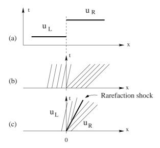
**Fig. 2.14.** (a) Expansive discontinuous initial data (b) picture of characteristics and (c) rarefaction shock solution on *x-t* plane
