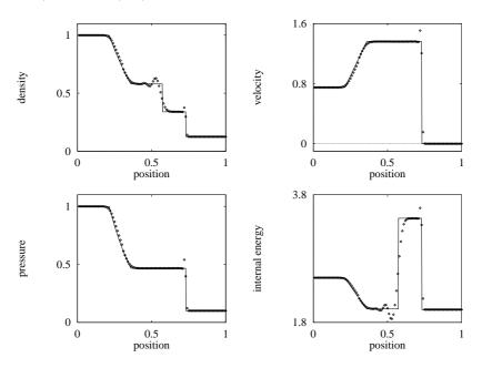
Fig. 6.18. The Richtmyer method applied to Test 1, with  $x_0 = 0.3$ . Numerical (symbol) and exact (line) solutions are compared at the output time 0.2 units
