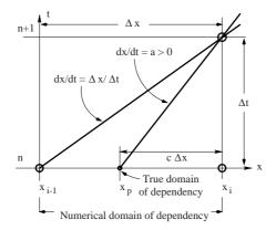
**Fig. 5.3.** Stencil of first–order upwind scheme (CIR) for positive speed a of wave propagation. Upwind direction lies on the left hand side.
