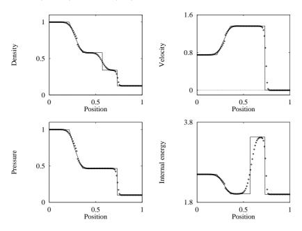
Fig. 8.4. Van Leer FVS scheme applied to Test 1, with  $x_0 = 0.3$ . Numerical (symbol) and exact (line) solutions are compared at time 0.2 units
