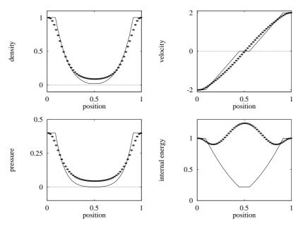
**Fig. 6.14.** The Lax–Friedrichs method applied to Test 2, with  $x_0 = 0.5$ . Numerical (symbol) and exact (line) solutions are compared at the output time 0.15 units
