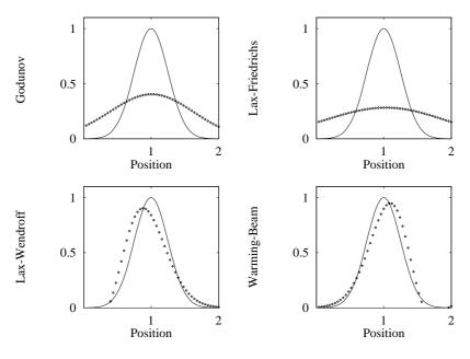
Fig. 5.10. Test 1: Comparison of numerical results for four numerical schemes (symbols) with the exact solution (line) at time 10 units (1250 time steps)
