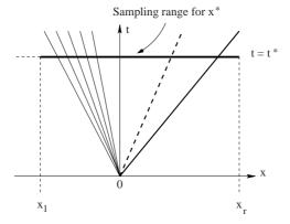
**Fig. 7.3.** Spacial sampling range in the solution of the Riemann problem at a given time  $t=t^*$
