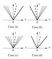
**Fig. 4.2.** Possible wave patterns in the solution of the Riemann problem: (a) left rarefaction, contact, right shock (b) left shock, contact, right rarefaction (c) left rarefaction, contact, right rarefaction (d) left shock, contact, right shock
