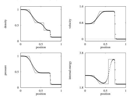
Fig. 7.18. FORCE scheme applied to Test 1, with  $x_0 = 0.3$ . Numerical (symbol) and exact (line) solutions are compared at the output time 0.2 units
