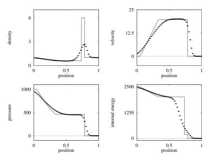
Fig. 6.15. The Lax–Friedrichs method applied to Test 3, with  $x_0 = 0.5$ . Numerical (symbol) and exact (line) solutions are compared at the output time 0.012 units
