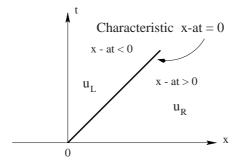
Fig. 2.3. Illustration of the solution of the Riemann problem in the x-t plane for the linear advection equation with positive characteristic speed a
