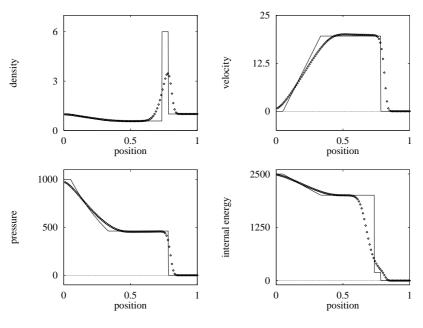
Fig. 7.20. FORCE scheme applied to Test 3, with  $x_0 = 0.5$ . Numerical (symbol) and exact (line) solutions are compared at the output time 0.012 units
