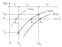
Fig. 4.6. Behaviour of the pressure function in the solution of the Riemann problem
